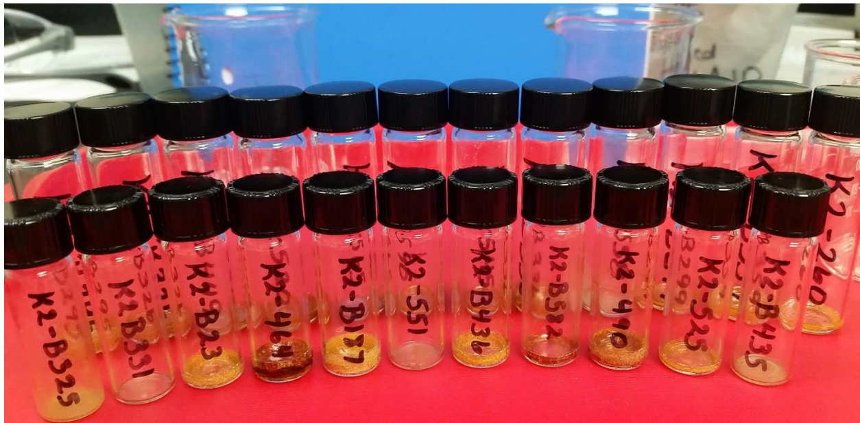
Figure 7: Photograph of dried collagen in glass dram vial ready to be weighed for isotopic processing.
