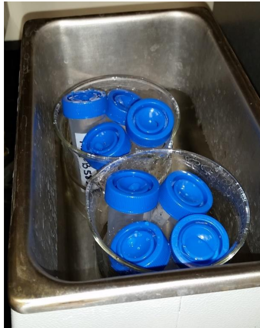
Figure 4: Photograph of samples being cleaned by ultrasonication.
